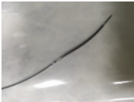
Fig.-1: Image shows the deformed distal end of stent balloon showing stent strut fracture
